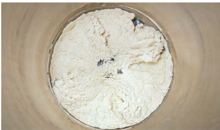
Advanced design of bottom agitator guarantees optimal powder flow into the dosing screw even for very cohesive powders
